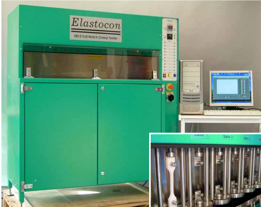
Full Notch Creep Tester (FNCT)
