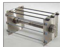
Tension Set Rig EV 04 , according to ISO 2285.
